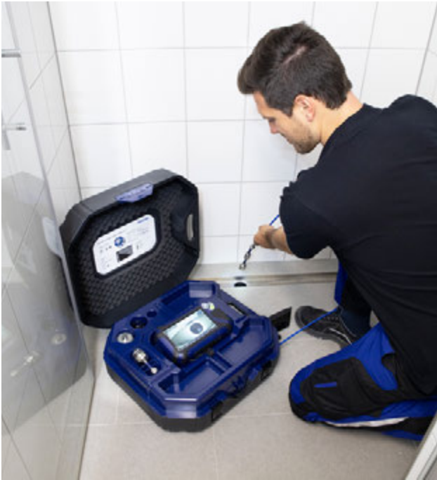
The waterproof camera head enables the inspection of sewers, among other things.
