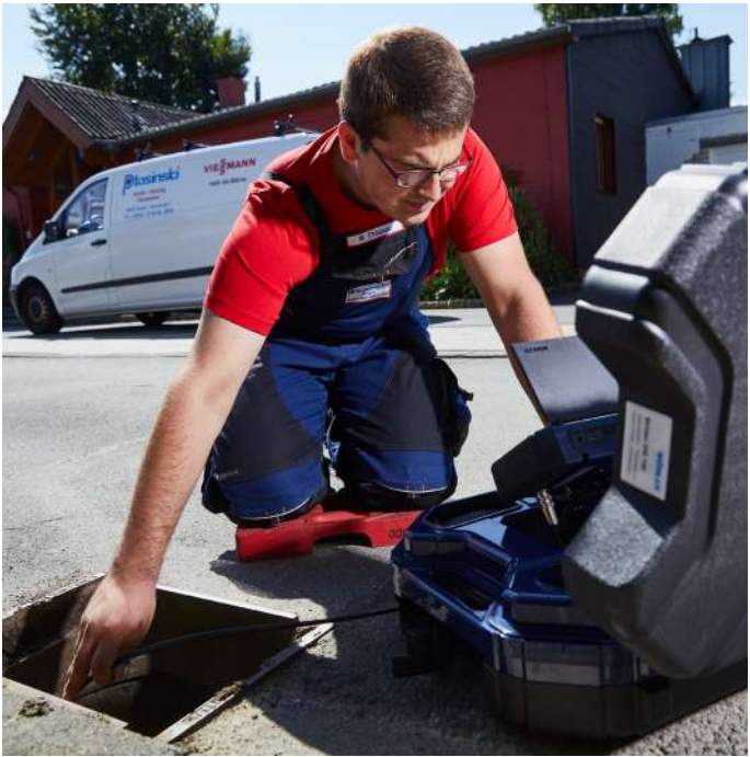
The waterproof camera head enables the inspection of waste water channels, among other things. The integrated anti-glare protection ensures the best view of the monitor even in strong sunlight.
