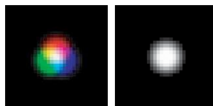
Composite images produced from conventional filter sets (above left), which typically have significant pixel shift, are distorted, whereas BrightLine ZERO pixel shift filter sets (above right) yield precise multi-color images.
