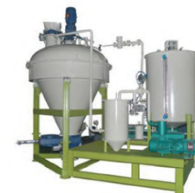
▶ 真空油脂噴塗機 (12~25% 增油量) Vacuum oil coating device (12~25% oil add)
